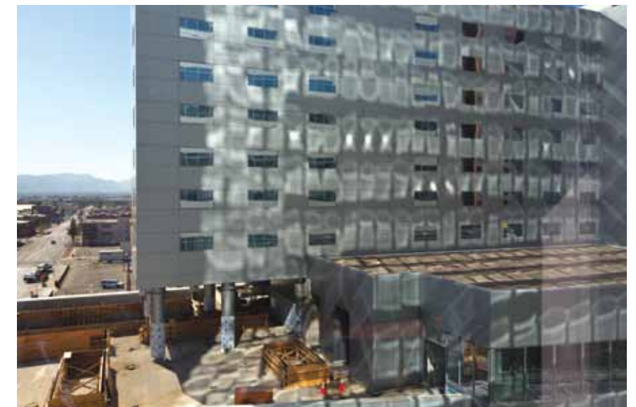
CITYSCAPE LOOKING SOUTH: Reflected light from a mirrored glass and steel structure tracks across the side of the City of Phoenix Transit office. Related temperature data proves a heat increase of between ten to 15 degrees.
